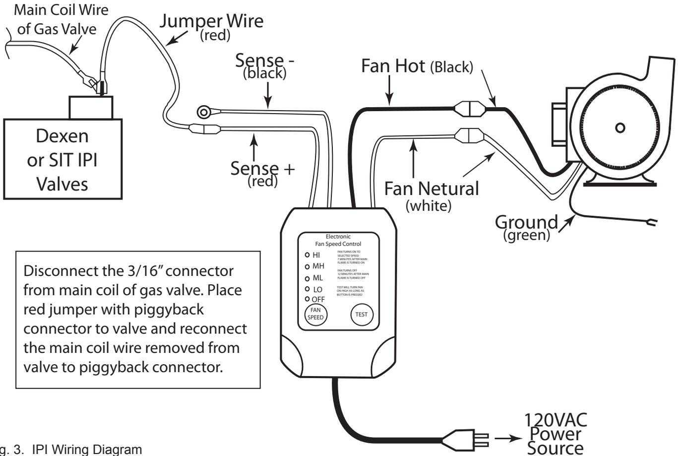
Fig. 3. IPI Wiring Diagram
