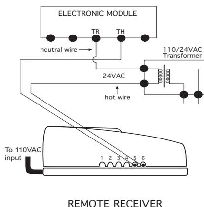
The remote control receiver can be connected, in series, to a 24VAC transformer to the TR (transformer) terminal on the ELECTRONIC MODULE. Connect the hot wire from the 24VAC transformer to either of the wires on the remote receiver. Connect the other wire from the receiver to the TH (thermostat) terminal on the ELECTRONIC MODULE.
